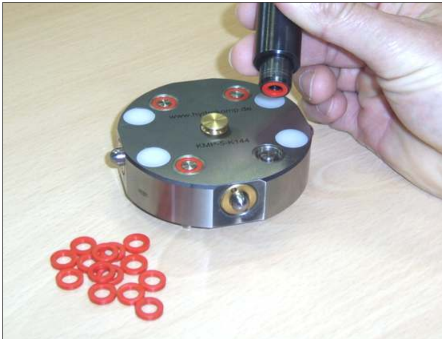
Mounting tool with inserted system seal prior to pressing into the coupling mechanism
